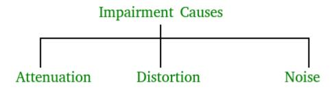
Attenuation – It means loss of energy. The strength of signal decreases with increasing distance which causes loss of energy in overcoming resistance of medium. This is also known as attenuated signal. Amplifiers are used to amplify the attenuated signal which gives the original signal back and compensate for this loss.
